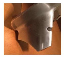
First it is necessary to identify the lowest point of the allowable hole, which is 1.500" below the flat area of the cavitation plate. It is important to ensure that you are measuring outside the radius at the bottom of the exhaust strut. Using a ruler, mark the leading edge of the strut and draw a line parallel to the cavitation plate. This line is the maximum limit of the hole.
