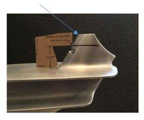
Using a business card, align the bottom edge of the card with the edge of the water inlet hole and the long edge of the card with the leading edge of the exhaust strut. Holding the card with one hand, use a Sharpie to draw a line for the edge of the exhaust strut, leading downward to the cavitation plate. This line represents the angle at which the water inlet hole would be enhanced.
